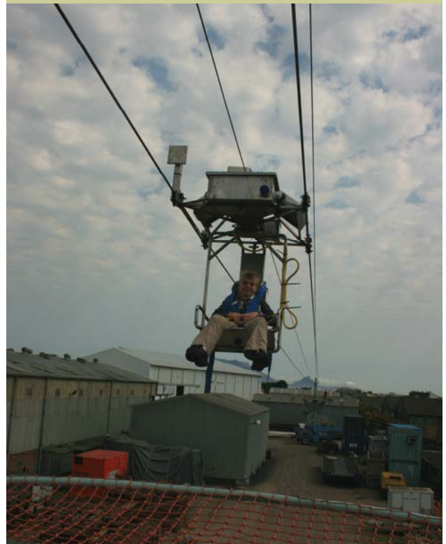
AERIAL ROPEWAY SYSTEM PERSONNEL TRANSFER BETWEEN TOWERS DURING COMMISSIONING.
