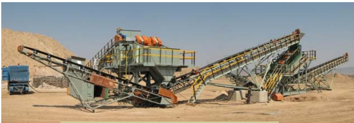
A MOBILE DRY IN-FIELD SCREENING (DIFS) PLANT AT DABERAS
