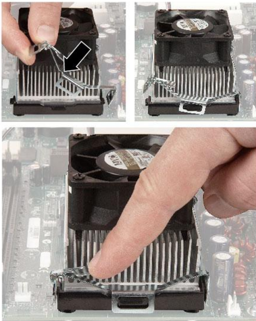
Heat sink with removable retention clips
