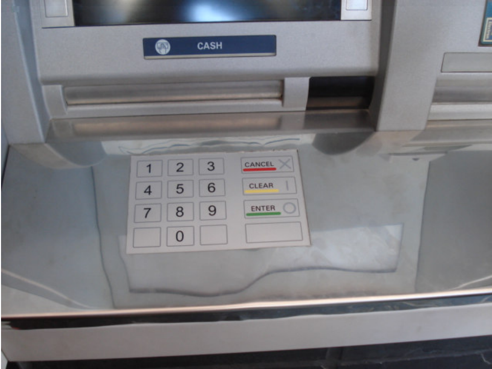
Figure 9: Fake keypad on top of genuine keypad
