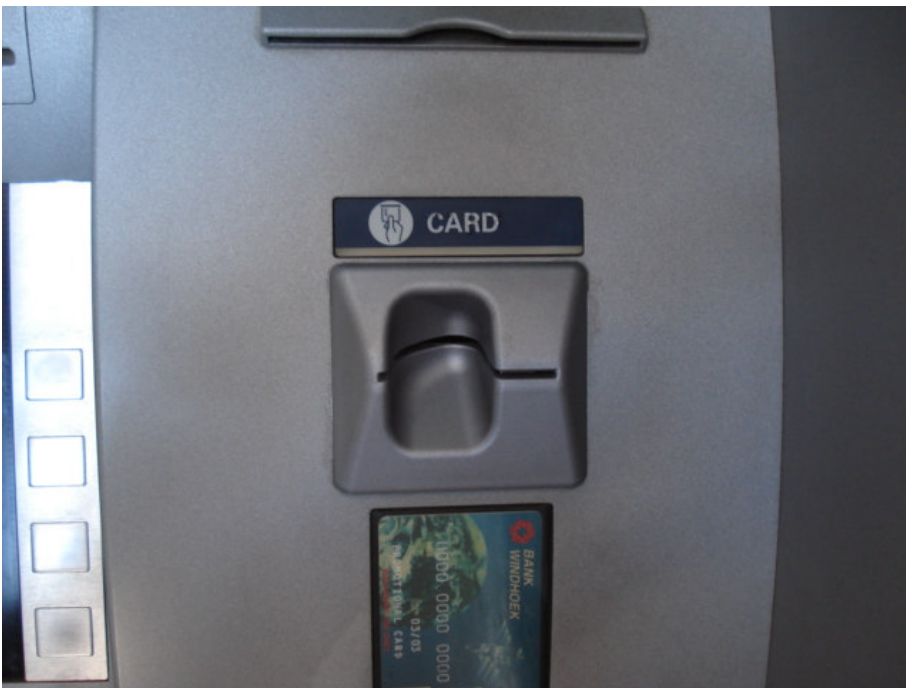
Figure 4: Skimmer device in the Card slot
