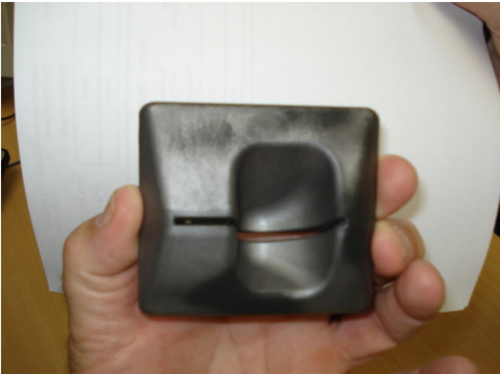
Figure 6: Card Reader "skimmer device"
