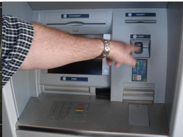
Figure 2: Card Reader Skimmer Device on ATM
