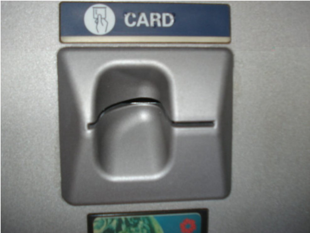
Figure 5: Closer look at the Skimmer device in Card slot
