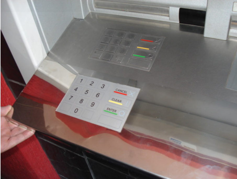
Figure 11: False face fit over Keypad
