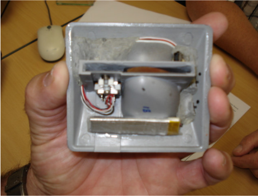
Figure 7: Storage and transmitting devices on the back of the Card Skimmer
