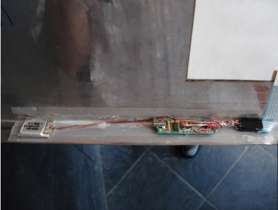
Figure 13: Storage or transmitting device on the back of the false plate
